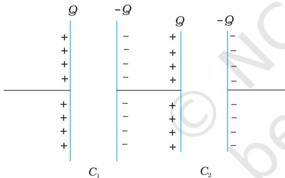
FIGURE 2.26 Combination of two capacitors in series.
