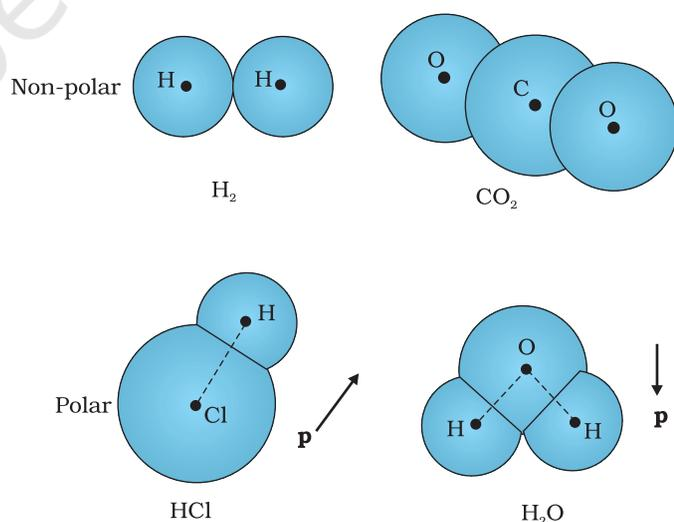
**FIGURE 2.21** Some examples of polar and non-polar molecules.
