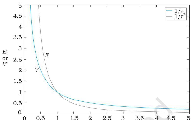
**FIGURE 2.4** Variation of potential  $V$  with  $r$  [in units of  $(Q/4\pi\epsilon_0) \text{ m}^{-1}$ ] (blue curve) and field with  $r$  [in units of  $(Q/4\pi\epsilon_0) \text{ m}^{-2}$ ] (black curve) for a point charge  $Q$ .
