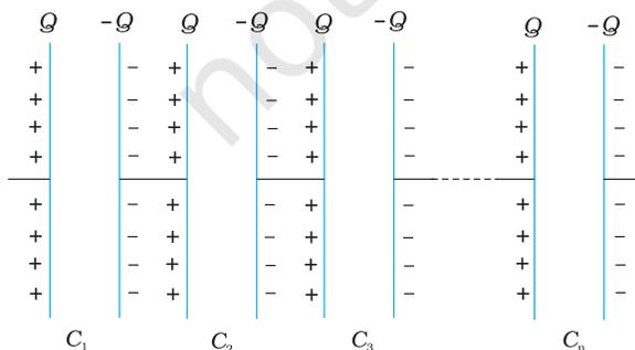
FIGURE 2.27 Combination of  $n$  capacitors in series.
