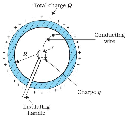
**FIGURE 2.32** Illustrating the principle of the electrostatic generator.
