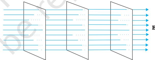
**FIGURE 2.10** Equipotential surfaces for a uniform electric field.
