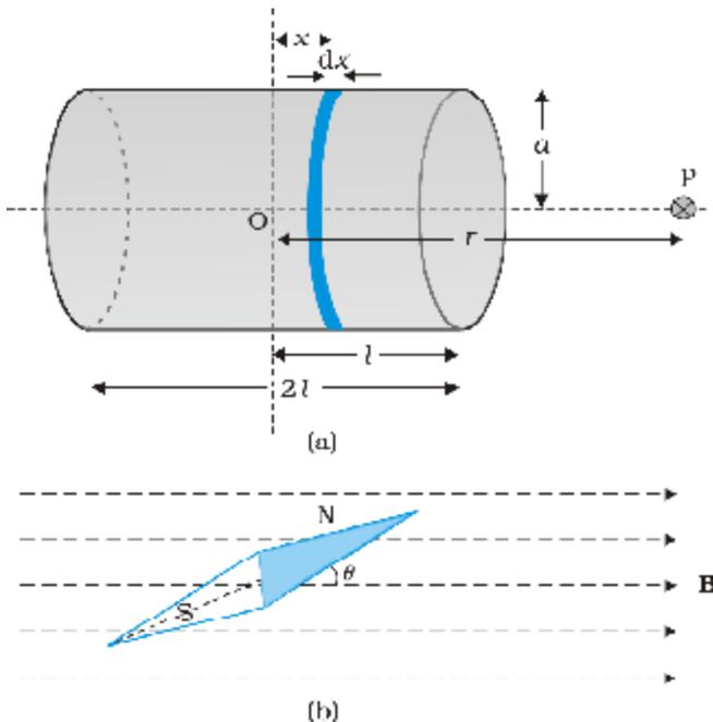
FIGURE 5.4 Calculation of (a) The axial field of a finite solenoid in order to demonstrate its similarity to that of a bar magnet. (b) A magnetic needle in a uniform magnetic field  $B$ . The arrangement may be used to determine either  $B$  or the magnetic moment  $m$  of the needle.
