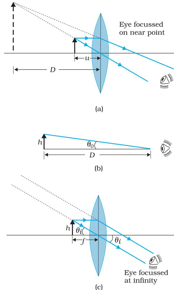
**FIGURE 9.30** A simple microscope; (a) the magnifying lens is located such that the image is at the near point, (b) the angle subtended by the object, is the same as that at the near point, and (c) the object near the focal point of the lens; the image is far off but closer than infinity.
