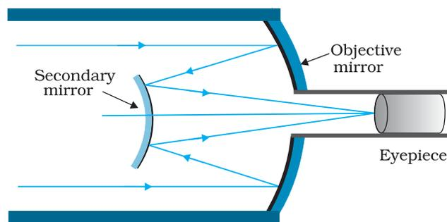
FIGURE 9.33 Schematic diagram of a reflecting telescope (Cassegrain).
