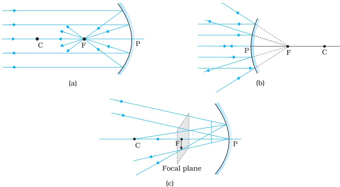
**FIGURE 9.3** Focus of a concave and convex mirror.
