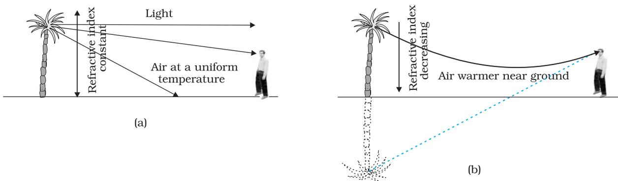
**FIGURE 9.14** (a) A tree is seen by an observer at its place when the air above the ground is at uniform temperature, (b) When the layers of air close to the ground have varying temperature with hottest layers near the ground, light from a distant tree may undergo total internal reflection, and the apparent image of the tree may create an illusion to the observer that the tree is near a pool of water.
