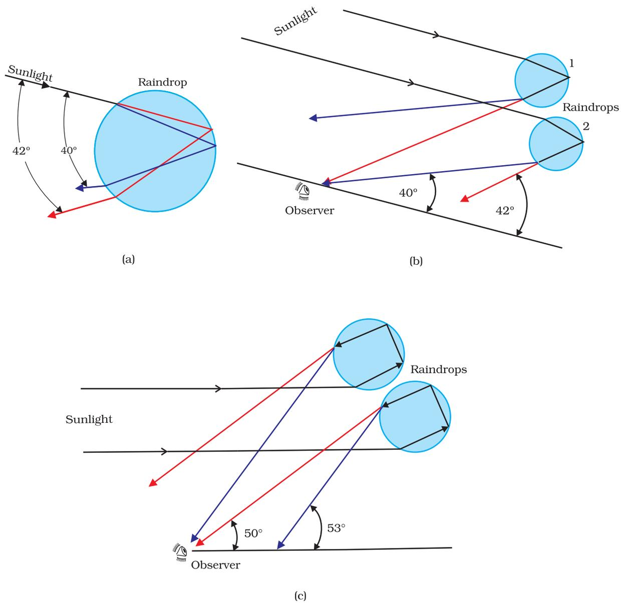
**FIGURE 9.27** Rainbow: (a) The sun rays incident on a water drop get refracted twice and reflected internally by a drop; (b) Enlarge view of internal reflection and refraction of a ray of light inside a drop form primary rainbow; and (c) secondary rainbow is formed by rays undergoing internal reflection twice inside the drop.
