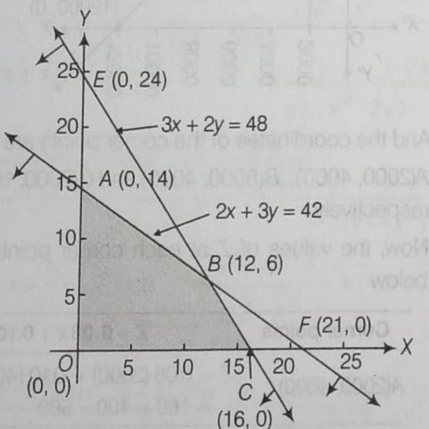
From the graph, OABCD is the feasible region which is bounded. The corner points are O(0, 0), A(0, 14), B(12, 6) and C(16, 0).
