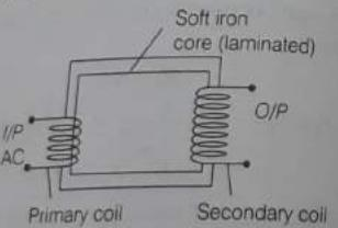
Working When alternating current source is connected to the ends of primary coil, the current changes continuously in the primary coil, due to which the magnetic flux linked with the secondary coil changes continuously. Therefore, the alternating emf of same frequency is developed across the secondary coil. [2]
