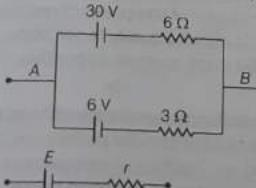
where,  $E$  = emf or potential of cells in parallel combination
