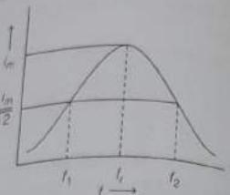
Half power frequencies are the frequencies on either side of resonant frequency for which current reduces half of its maximum value. In the above figure,  $f_1$  and  $f_2$  are half power frequencies.
